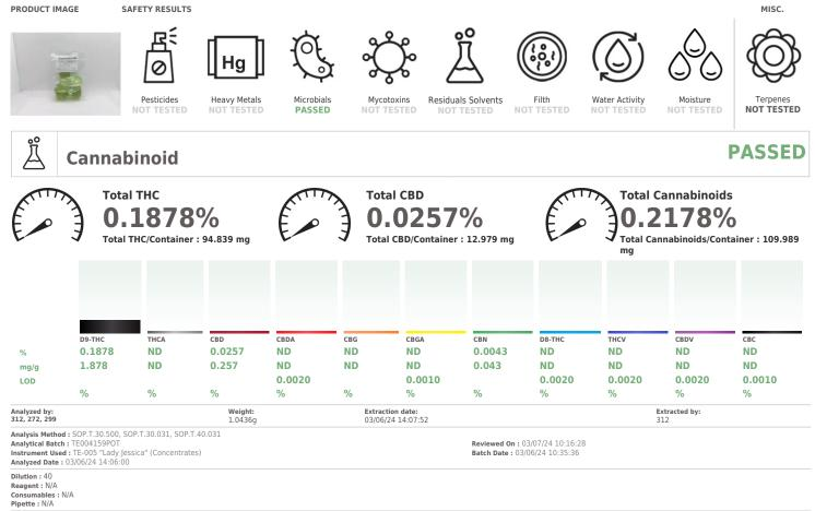
Full spectrum cannabinoid analysis utilizing High Performance Liquid Chromatography with Photo Diode Array detector (HPLC-PDA) for analysis. (Methods: SOP.T.30.500 for sample homogenization, SOP.T.30.031 for sample prep, SOP.T.40.031 for analysis on Shimadzu LC-2DX0 series HPLCs). Potency results for cannabis flower products are reported on an "as received" basis. without moleture correction.
